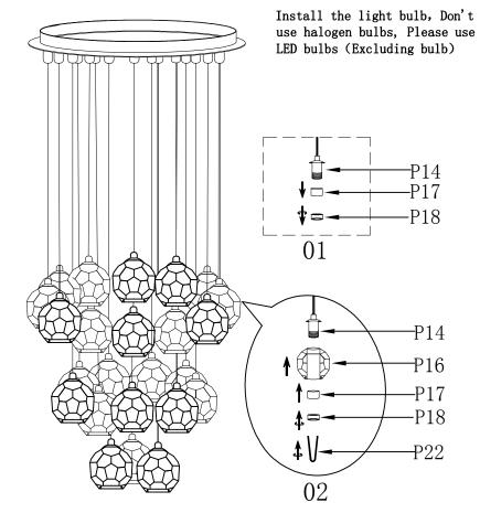
01. Unscrew the lamp holder ring (P18) counterclockwise, and then remove the iron tube (P17);
